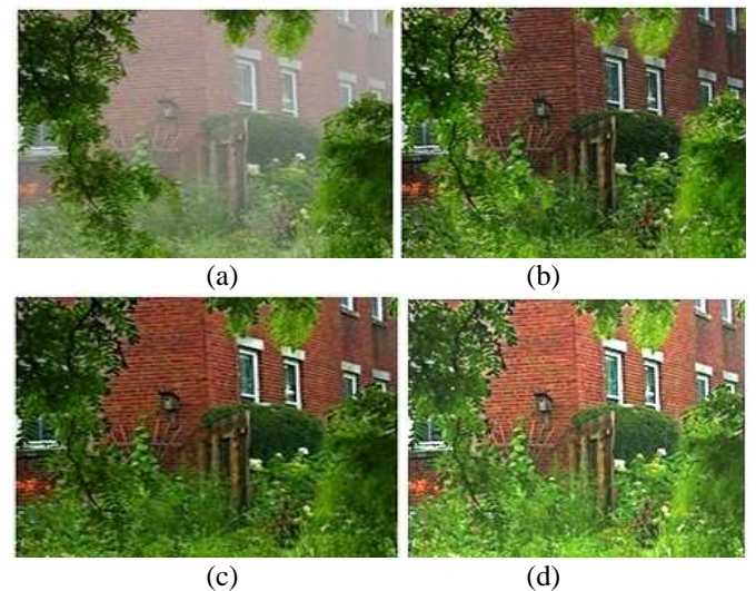
Fig. 5. Visual comparison of the dehazing results of these methods for a heavy foggy color image. These methods are [26, 9] and the proposed algorithm using image filtering approach. (a) Foggy image, (b) [26], (c) [9] (d) the proposed algorithm.
