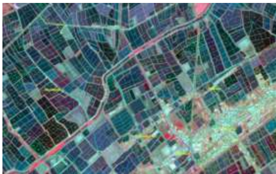
Fig.6. Cadastral Layer (Survey Numbers) superimposed on Aquaculture ponds in Krishna district as seen on IRS LISS-IV Satellite Image (Date-12th June 2014)
