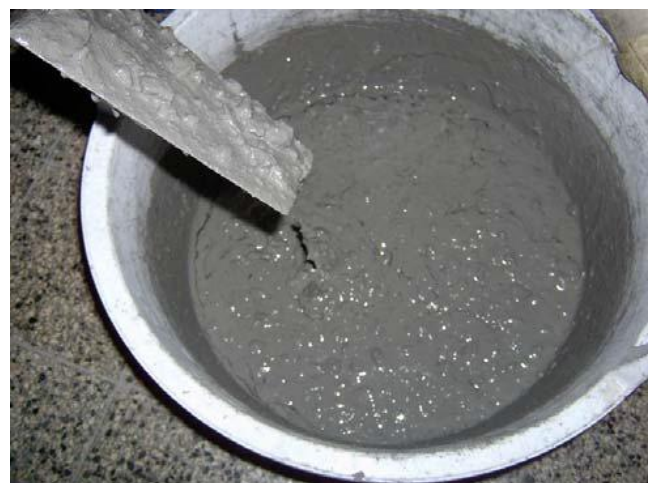
Fig.1: Freshly prepared geo-polymer concrete
