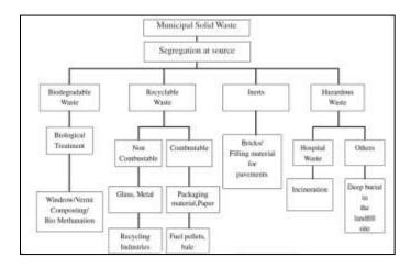
Figure 2: Schematic of solid waste segregation at source at Jabalpur
